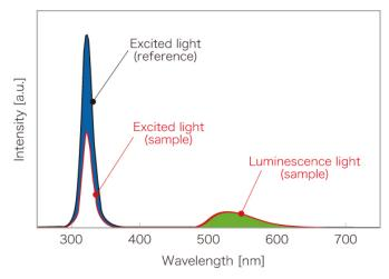
Excitation light on reference and sample and photoluminescence spectrum measurement
