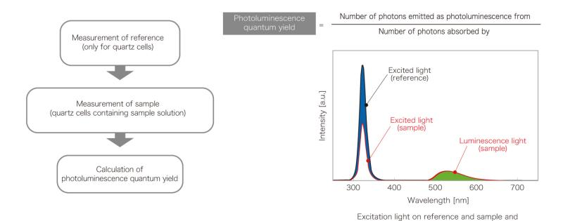
photoluminescence spectrum measurement
