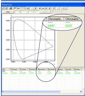
Besides displaying PL spectra and calculating quantum yields, the software also includes a function for color coordinates. Besides the chromaticity coordinates (x, y) of the measured sample, the three stimulus values (X, Y, Z) are displayed.
